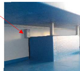
Power supply 12 v under the pan behind the cowl, to connect the scale
