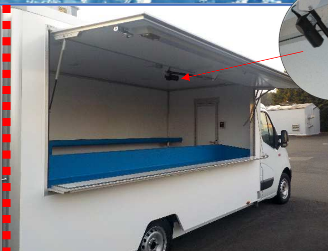
Side cowl and shelf, opening with gas springs and central electric cylinder – special profile for 90° locking of the shelf
