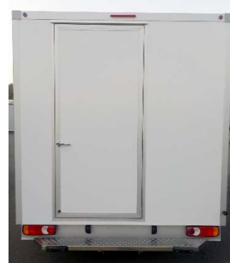
Eccentric rear single door, int/ext handle with key lock, 180° magnetic door retainer
