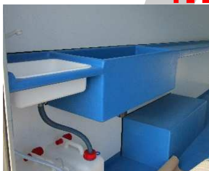
Desk on left side length, with plastic washer (+ 2 jerrycans, spout and submersible pump 12V), sink for mussels
